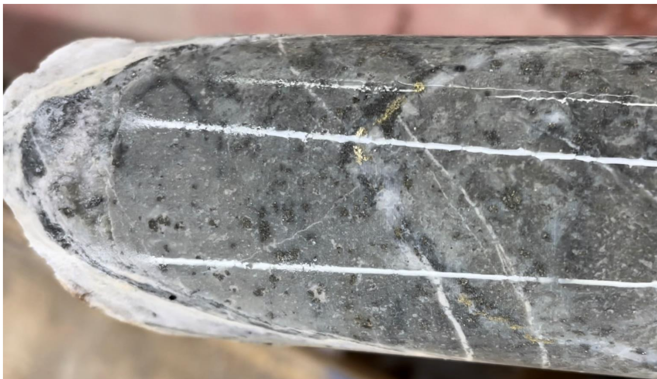
Figure 3 – Visible gold in hole P22-2445 in the 1.0m interval starting at a depth of 113.00m and grading 90.70 g/t Au and 19.75 g/t Ag
