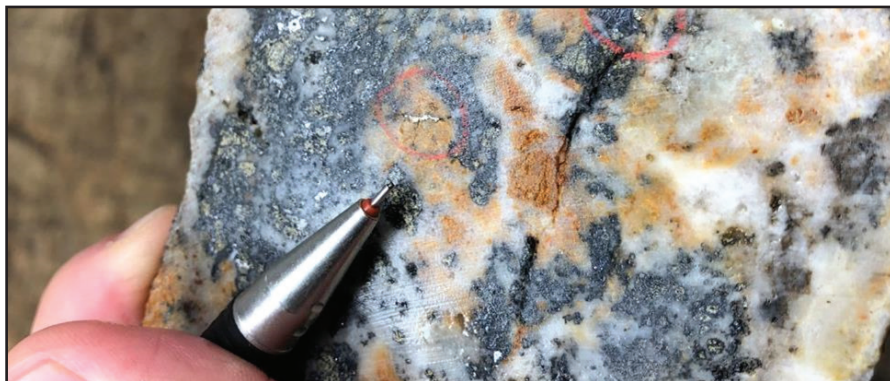
Image of a grab sample from the Silver Hill showing north of Long Lake. Sulfide mineralization and quartz are clearly visible. The red circles highlight grains that have been visually identified as electrum (alloy of gold and silver).
